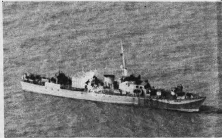
Large, stacked type is 110-ft. Fairmile subchaser, converted for long-range rescue missions and called RML (rescue motor launch). It has a low stack and bridge, with prominent deckhouse aft enclosing sick bay.
